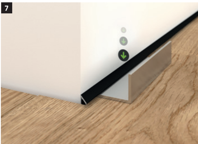
As soon as the clamping process is completed, the end profile is pressed down and the assembly aid is removed. Now the tensioning and assembly process is repeated until all assembly clips on an end profile are tensioned and countersunk. For any corrections the end profile can be removed from the connection joint at any time.
